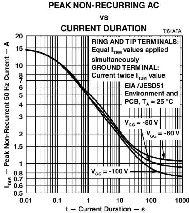
Figure 2. Non-repetitive Peak On-State Current against Duration
