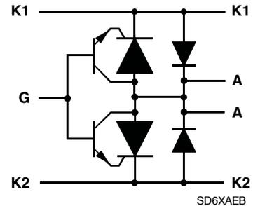
**D Package Top View and Device Symbol for Shunt (SD) Pin-Out**
