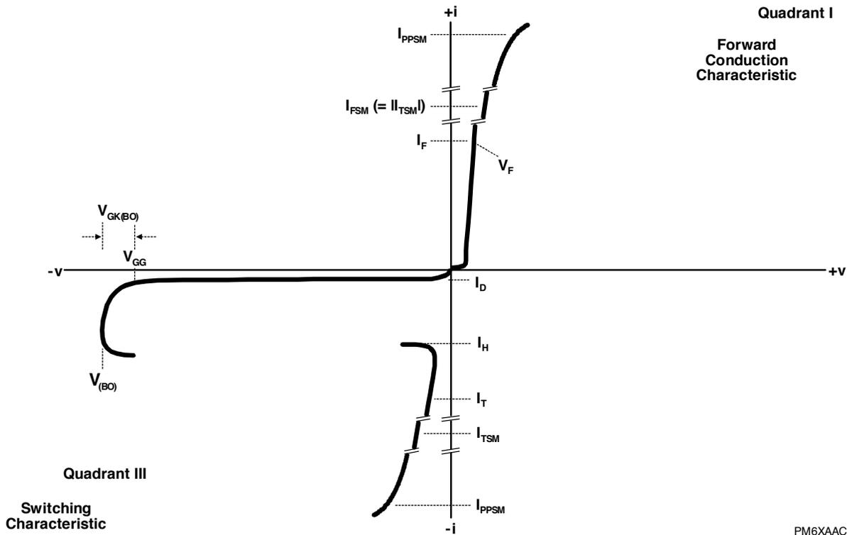
Figure 1. Voltage-Current Characteristic
