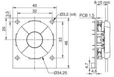
\*When the 1ZB is activated the diameter changes from 34,25mm to 35,0mm
