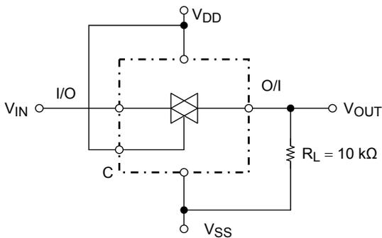
$$R_{ON} = 10 \times \frac{(V_{IN} - V_{OUT})}{V_{OUT}} [k\Omega]$$
