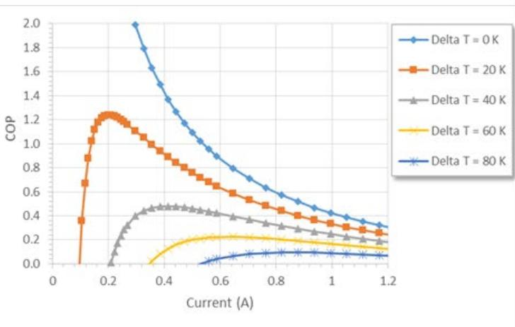
\*Note - Waste heat = Heat out of hot side
