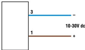
QD and cabled emitter hookups are functionally identical; black and white wires have no connection.
