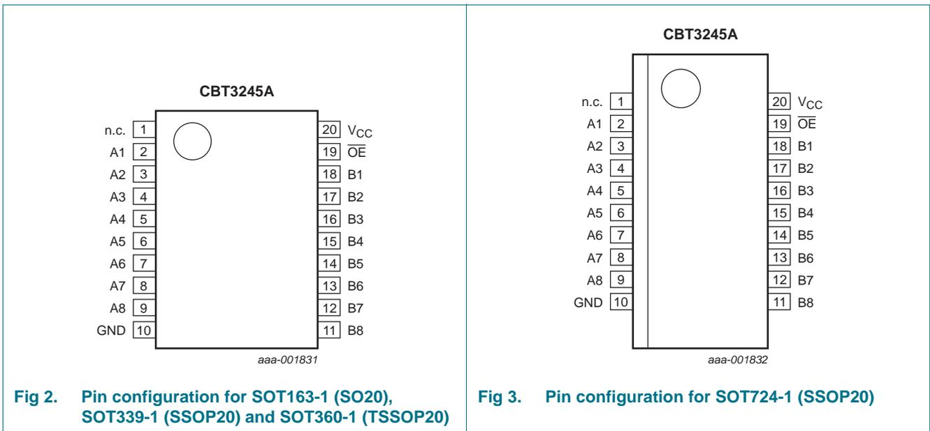
Fig 2. Pin configuration for SOT163-1 (SO20), SOT339-1 (SSOP20) and SOT360-1 (TSSOP20)
