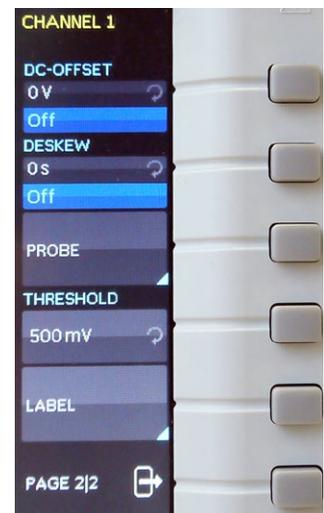
Fig. 2.10: Basic soft menu elements for settings and navigation
