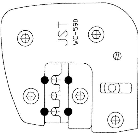
1. Open flap locator and insert contact up to stop.
