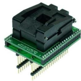
The conversion of this adapter is 1:1 (pin to pin). This adapter can be used with all chip programmers that support the desired chip and 1:1 adapters for it (the programmer must have at least a 44pin socket).
