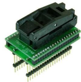
This adapter was designed specially for the BX40 and USB Chip programmer and can only be used with these devices.
