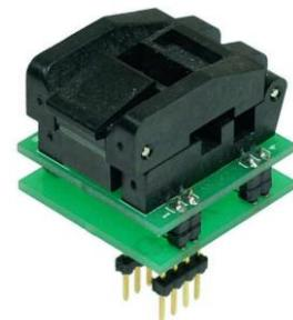
The conversion of this adapter is F:F (function to function). The adapter can be used for example for the BX32, BX32P, BX40 and Galep-4 programmers. With the Leaper-48 and the Superpro 3000U the adapter can only be used if the chip with the DIP8 package is selected in the respective software instead of the SOP14 package.
