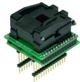
The conversion of this adapter is F:F (function to function). The adapter can be used for example for the BX32, BX32P and Galep-4 programmers. With the Leaper-48 and the Superpro 3000U the adapter can only be used if the chip with the DIP28 package is selected in the respective software instead of the PLCC32 package.
