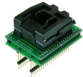
The conversion of this adapter is F:F (function to function). The adapter can be used for example for the Galep-4 programmers. With the Leaper-48 and the Superpro 3000U the adapter can only be used if the chip with the DIP40 package is selected in the respective software instead of the QFP44 package.
