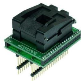
The conversion of this adapter is F:F (function to function). The adapter can be used for example for the BX40 and the Galep-4 programmers. With the Leaper-48 and the Superpro 3000U the adapter can only be used if the chip with the DIP40 package is selected in the respective software instead of the PLCC44 package.
