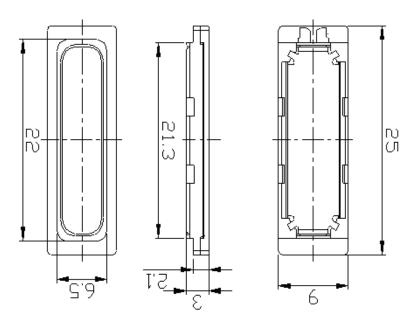
**6**Υ.Σ Meight 70~+82°C Storage temperature -30~+\0ec Operating temperature 10%Max Total harmonic distortion (at 1KHz/1W in 2cc box) 93±3dB Sound pressure level at 1.5kHz ZH000,02-01 Frequency range Resonant frequency V1/ZH%0Z±006 Maximum input power (for 1 min in 2cc box) WZ.1 W0.1 Rated input power Ω%31±8 Rated impedance (3KHz/1V) Specifications **ABS-240-RC**
