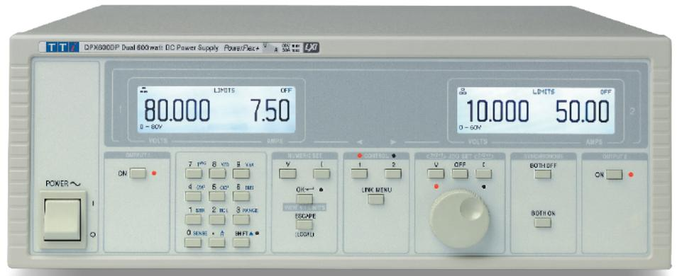
The QPX600D is a dual output dc power supply with a maximum total output power of 1200 watts and is suited to both bench-top and system applications. The QPX600DP incorporates full digital remote control using USB, RS-232, LAN and GPIB interfaces. Both models include analog remote control.
