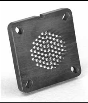
Headers provide easy separation of the connector from the PC board.
