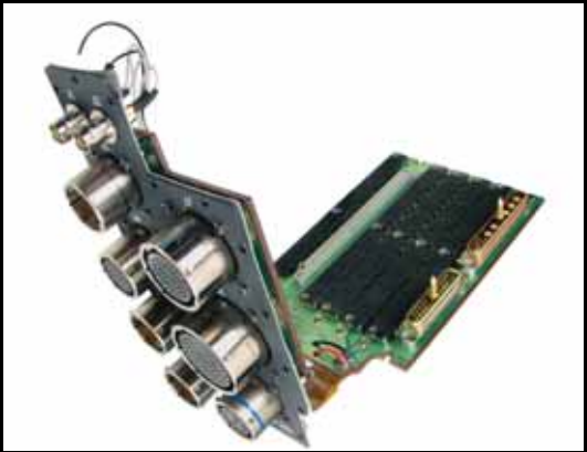
Backplane Assembly with LRM Connectors with Brush Contacts on one side and Cylindrical Connectors with Press-fit Compliant Contacts on the other.
