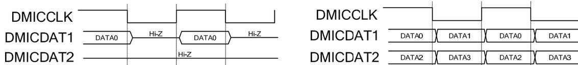
Figure 9 Digital Microphone Interface Protocol for One (left) or Four (right) Microphones
