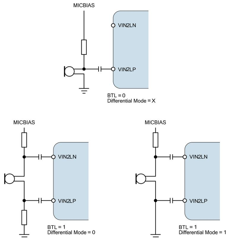
Figure 8 Port-B Example External Connections (one channel shown)
