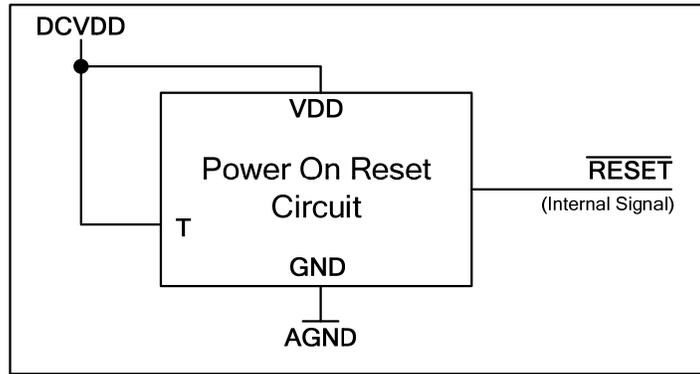
Figure 2 Internal Power on Reset Circuit Schematic
