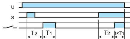
**(PE) Asymmetrical flasher (starting pulse off) with control signal - (Z1-Z2 linked).**
