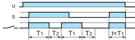
**(LE) Asymmetrical flasher (starting pulse on) with control signal - (Z1-Z2 open).**
