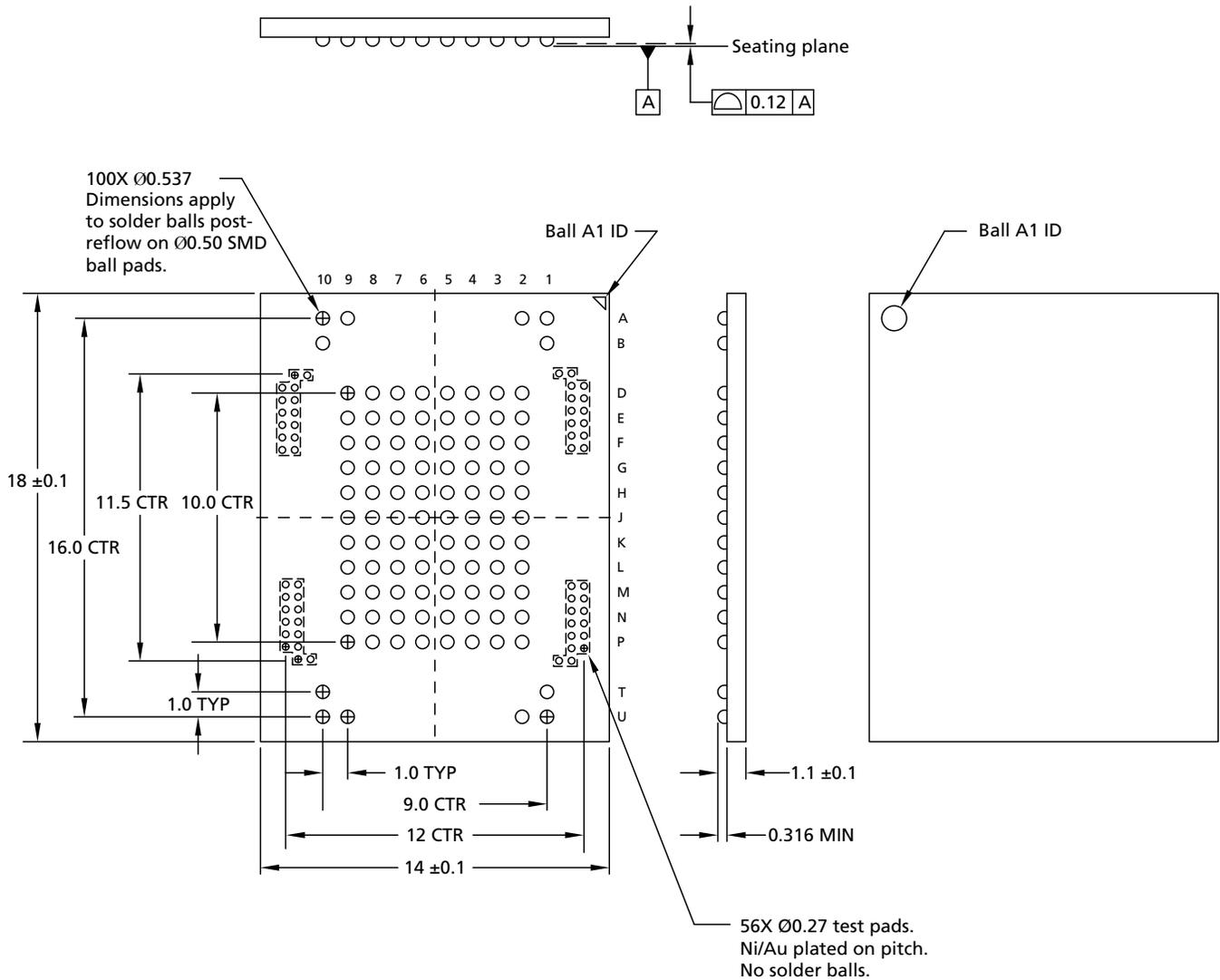
Note: 1. Dimensions are in millimeters.
