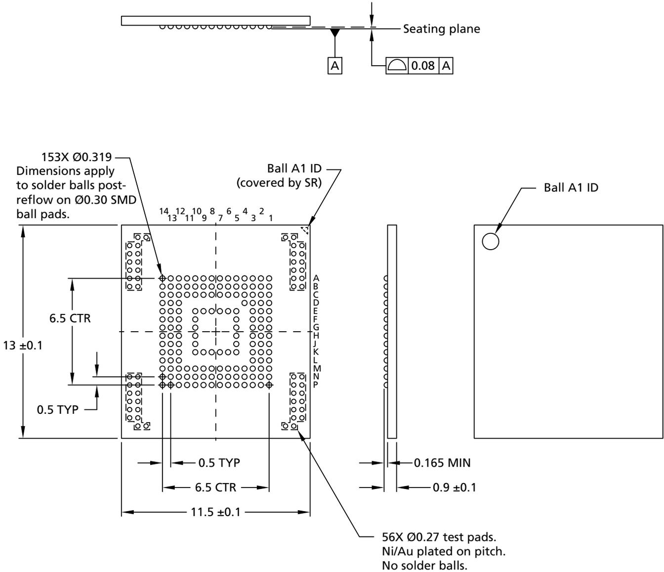
Note: 1. Dimensions are in millimeters.
