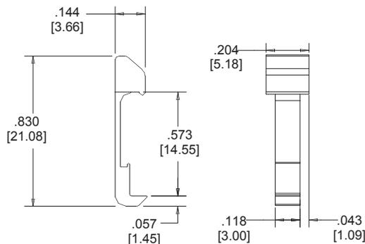
Note: Latches not compatible with reflow soldering. For reflow soldering, attach latches after soldering.
