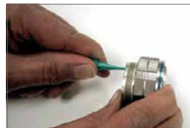
Plastic tool with contact in proper position.
