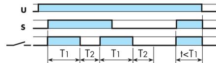
**(LE) Asymmetrical flasher (starting pulse on) with control signal**
