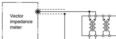
Vector impedance meter (YHP 4191A equivalent)
