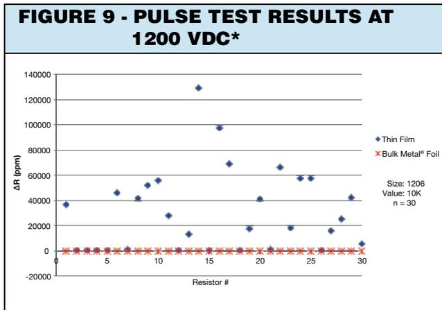
\* Note: Average of 30 units yielded deviation of 30,723 ppm of the Thin Film vs. -14 ppm for the Bulk Metal<sup>®</sup> Foil
