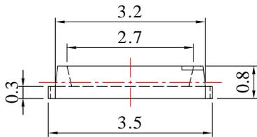
**Recommended Soldering Pad Dimensions**
