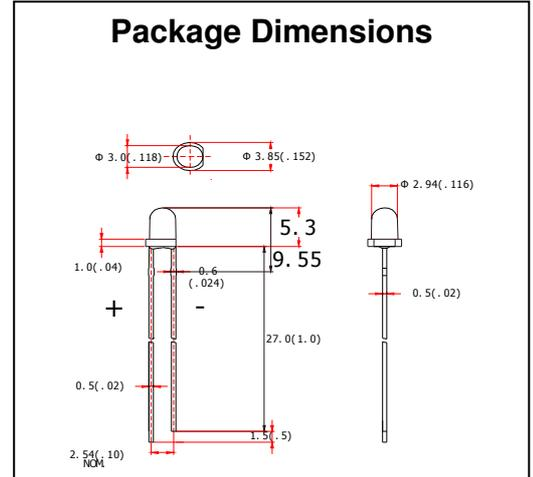
the LED chip was in reverse polarity, which is different from normal LED, please check the polarity of the LED before production. And please be noted that BIGGER side of the LED is "+ve"
