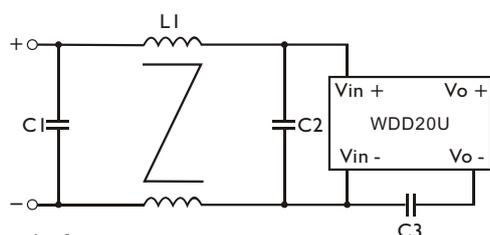
• Recommended EN 55022 Class B filter circuit layout.
