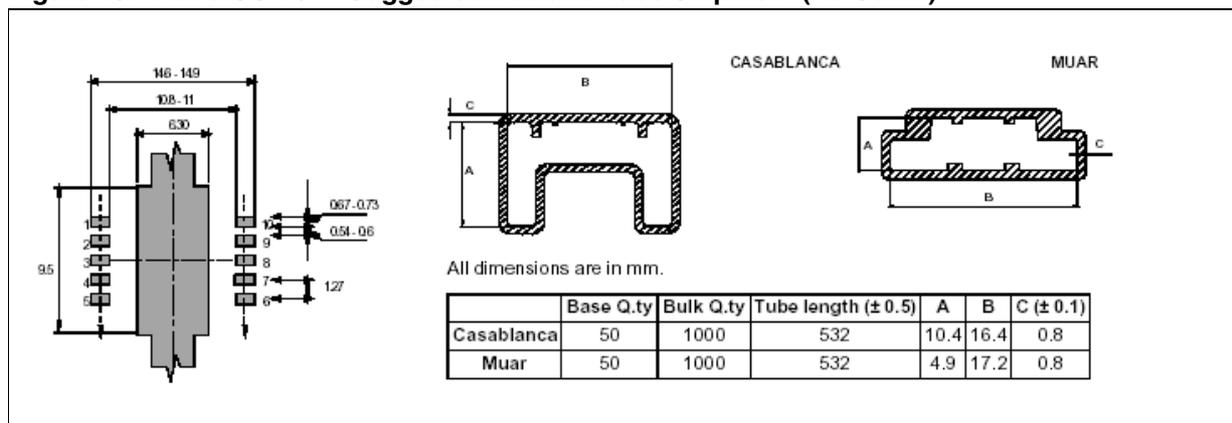
Figure 11. Tape and Reel Shipment (Suffix “TR“)
