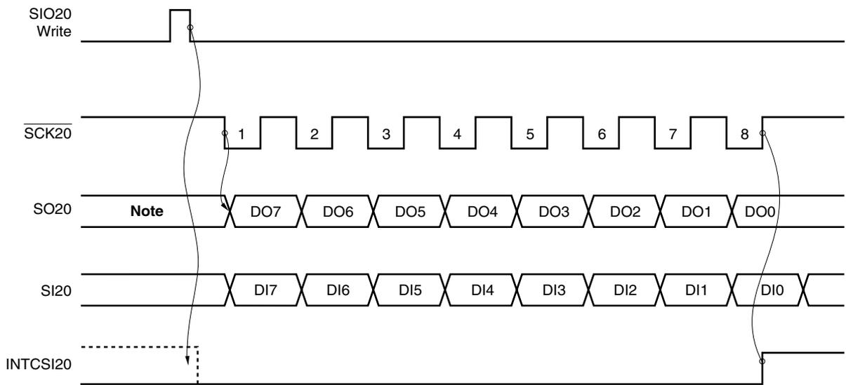
**Note** The value of the last bit previously output is output.
