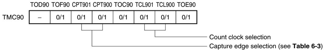
16-bit capture register 90 (TCP90) starts a capture operation after the CPT90 capture trigger edge is detected, and latches and retains the count value of 16-bit timer counter 90. TCP90 fetches the count value within 2 clocks and retains the count value until the next capture edge detection.
