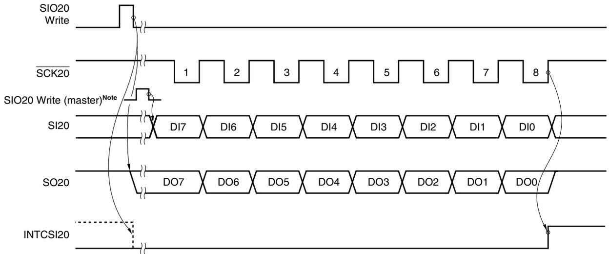
**Note** The data of SI20 is loaded at the first falling edge of  $\overline{\text{SCK20}}$ . Make sure that the master outputs the first bit before the first falling of  $\overline{\text{SCK20}}$ .
