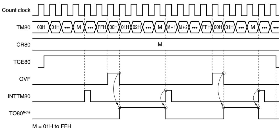
**Note** The initial value of TO80 is low when output is enabled (TOE80 = 1).
