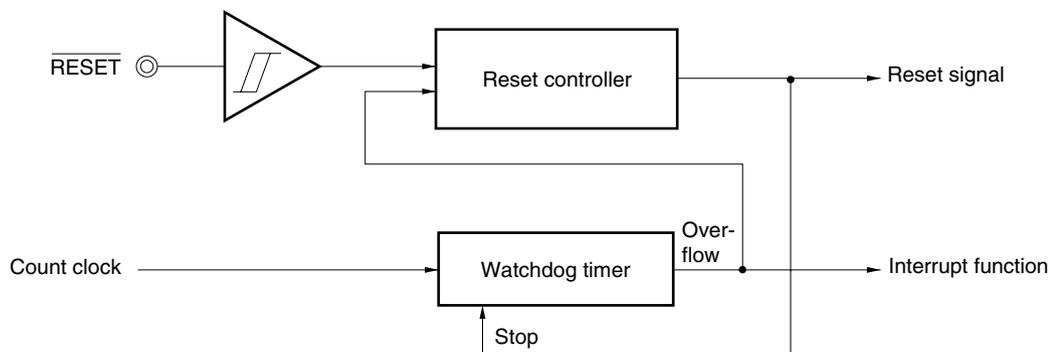
Figure 12-2. Reset Timing by  $\overline{\text{RESET}}$  Input
