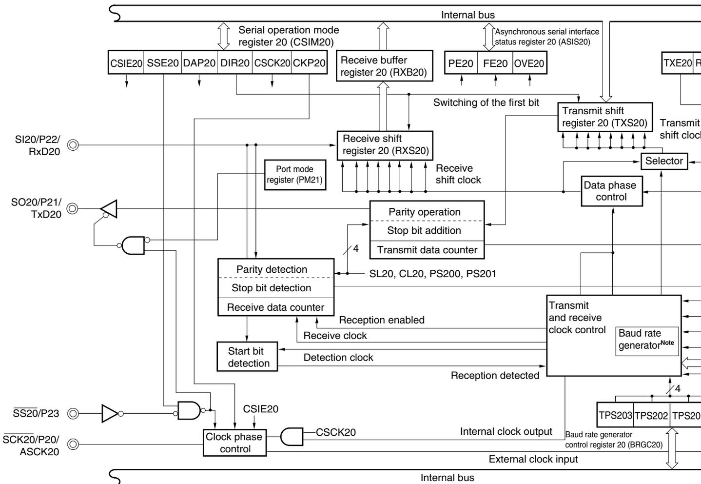
**Note** See Figure 9-2 for the configuration of the baud rate generator.
