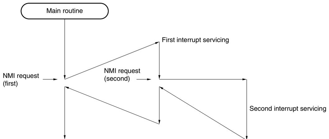
**10.4.2 Maskable interrupt request acknowledgment operation**
