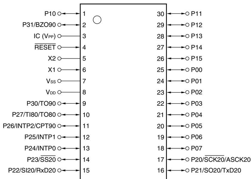
**Caution** Connect the IC (Internally Connected) pin directly to V<sub>ss</sub>.
