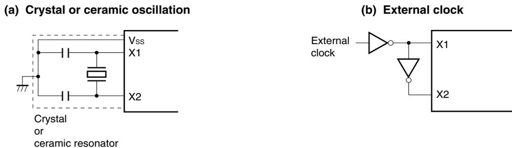
**Caution** When using the system clock oscillator, wire as follows in the area enclosed by the broken lines in Figure 5-3 to avoid an adverse effect from wiring capacitance.
