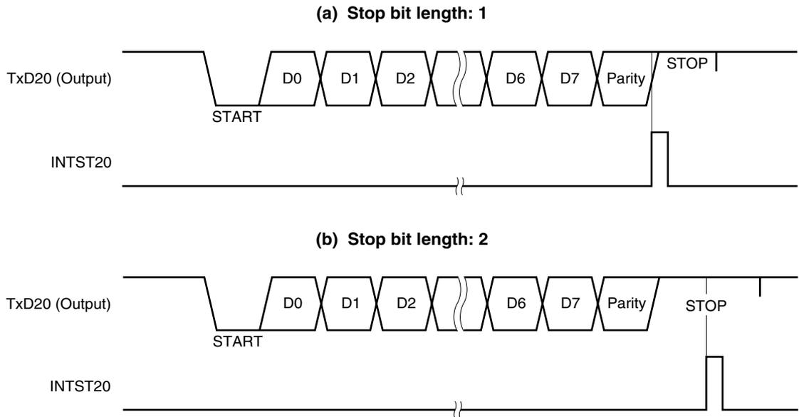
**Caution** Do not rewrite asynchronous serial interface mode register 20 (ASIM20) during a transmit operation. If the ASIM20 register is rewritten during transmission, subsequent transmission may not be performed (the normal state is restored by RESET input).
