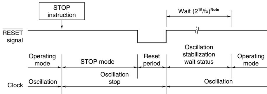
**Note** 3.28 ms (at  $f_x = 10.0$  MHz operation), 6.55 ms (at  $f_x = 5.0$  MHz operation)
