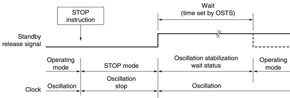
**Remark** The broken lines indicate the case where the interrupt request that has released standby mode is acknowledged.
