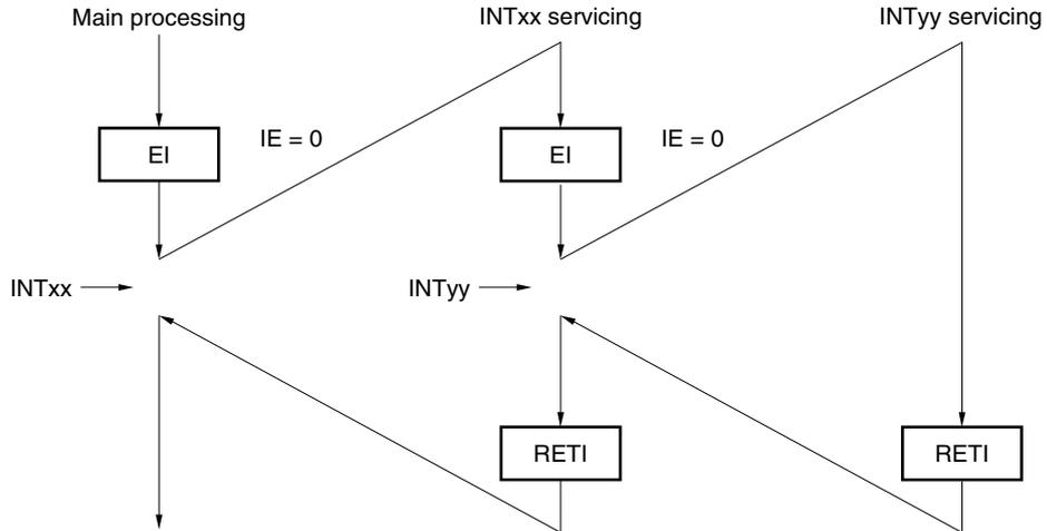
During interrupt INTxx servicing, interrupt request INTyy is acknowledged, and multiple interrupts are generated. The EI instruction is issued before each interrupt request acknowledgement, and the interrupt request acknowledgment enable state is set.
