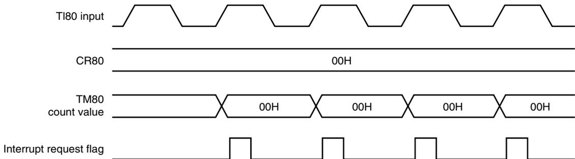
**Cautions 1.** Before rewriting CR80 in timer counter operation mode (PWME80 (bit 6 of 8-bit timer mode control register 80 (TMC80) = 0), stop the timer operation. If CR80 is rewritten while the timer operation is enabled, a match interrupt request signal may be generated immediately at the point of rewrite.
