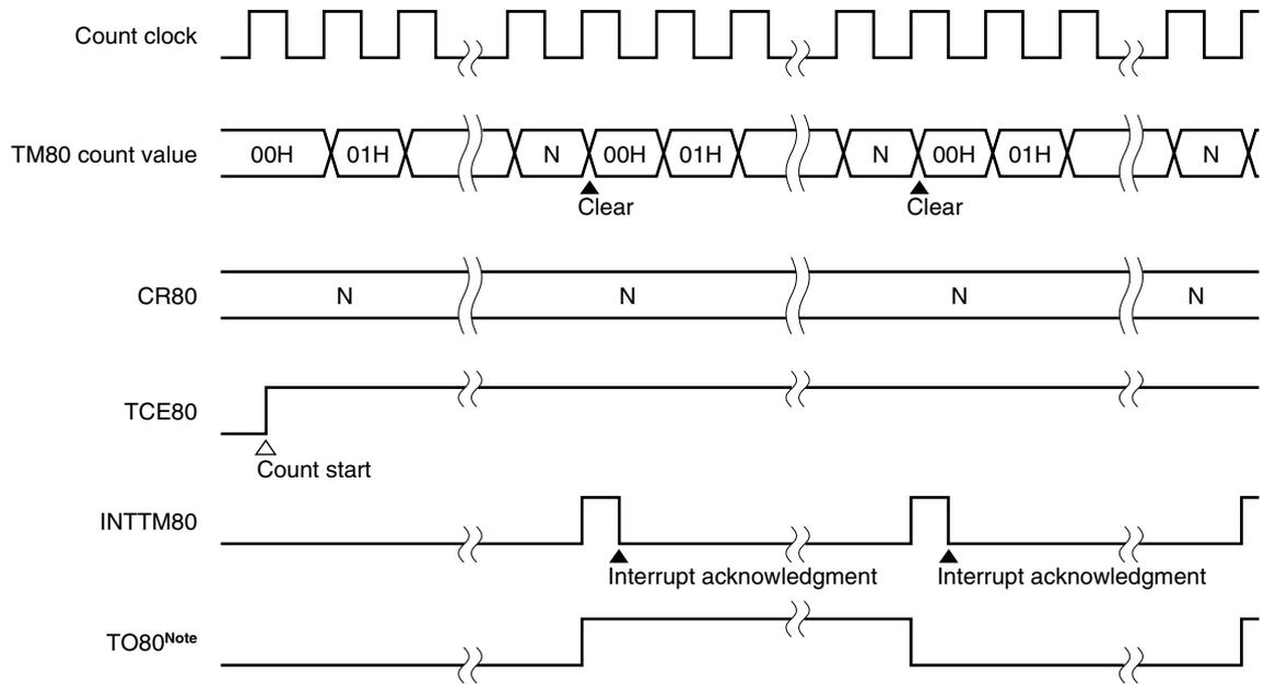
**Note** The initial value of TO80 is low when output is enabled (TOE80 = 1).
