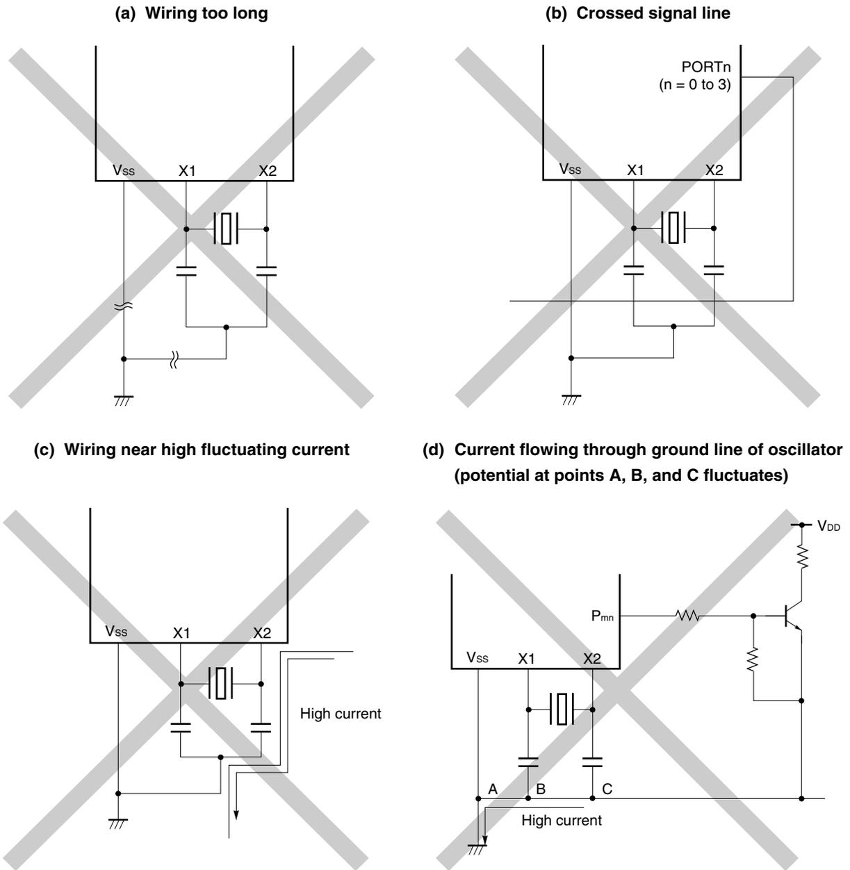
Figure 5-4. Examples of Incorrect Resonator Connection (2/2)
