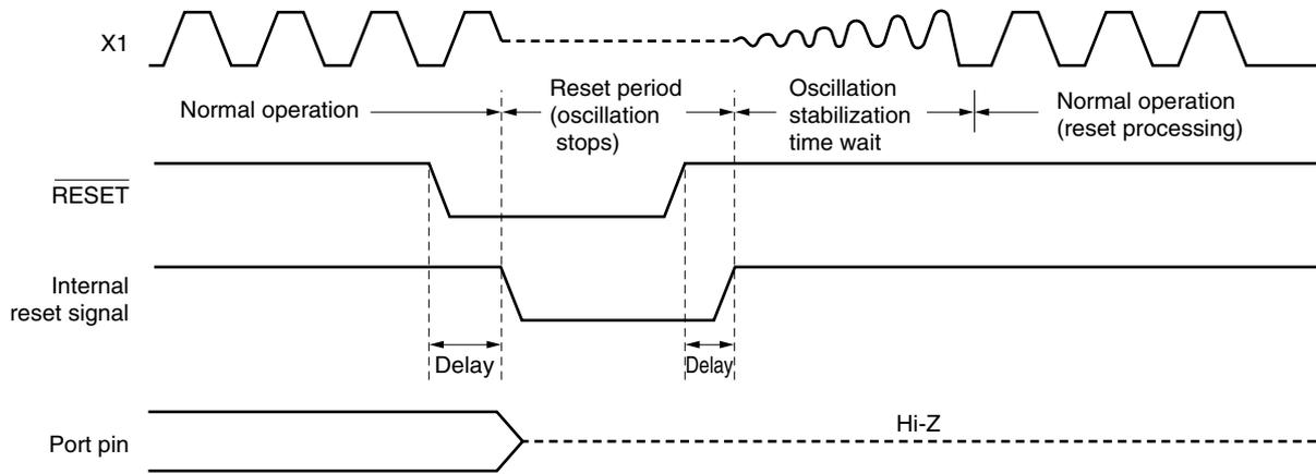
Figure 12-3. Reset Timing by Watchdog Timer Overflow
