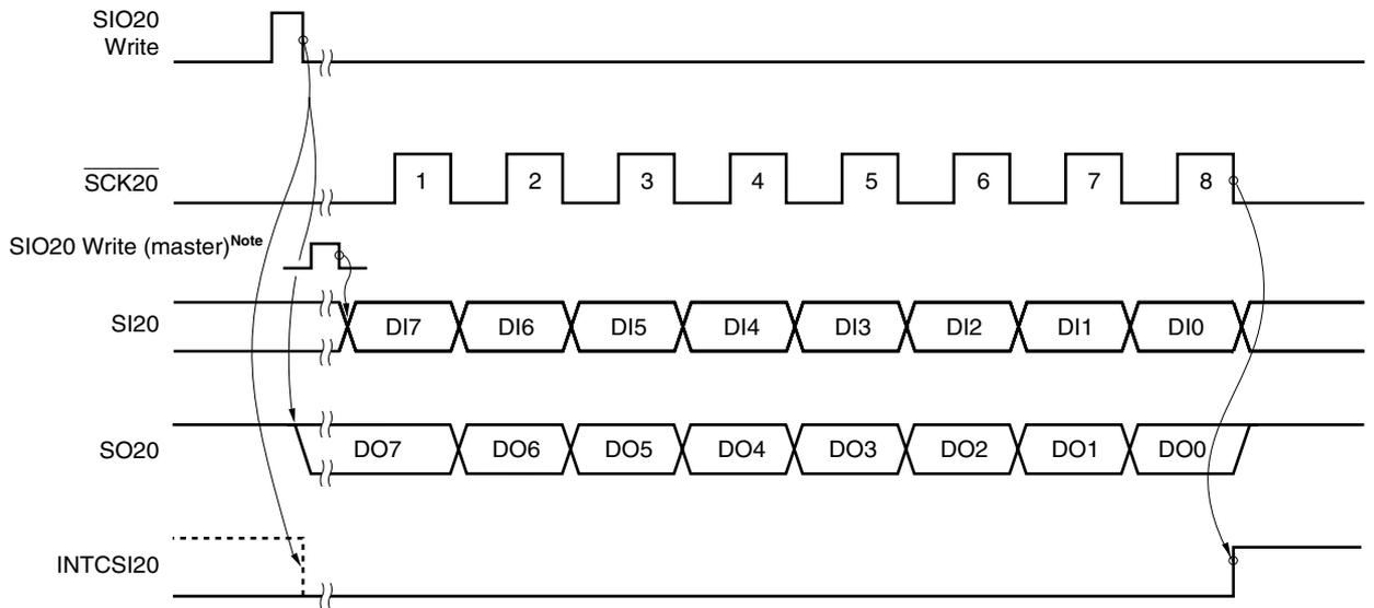
**Note** The data of SI20 is loaded at the first rising edge of SCK20. Make sure that the master outputs the first bit before the first rising of SCK20.
