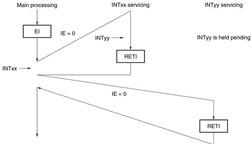
Because interrupts are not enabled in interrupt INTxx servicing (the EI instruction is not issued), interrupt request INTyy is not acknowledged, and multiple interrupts are not generated. The INTyy request is reserved and acknowledged after the INTxx servicing is performed.
