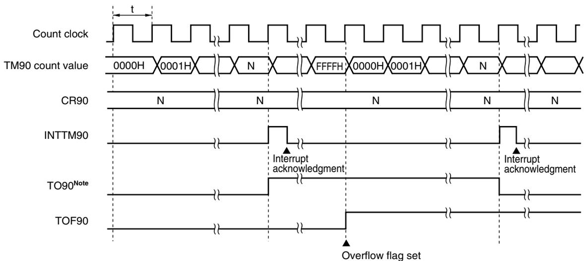
**Note** The TO90 initial value becomes low level during output enable (TOE90 = 1).
