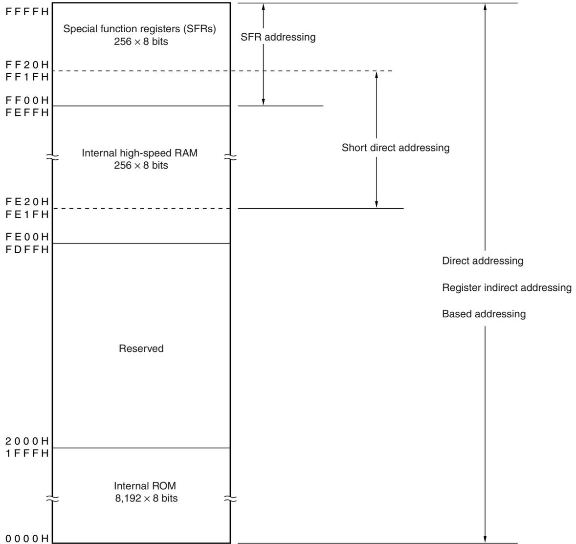
Figure 3-8. Data Memory Addressing ( $\mu$ PD78F9076)
