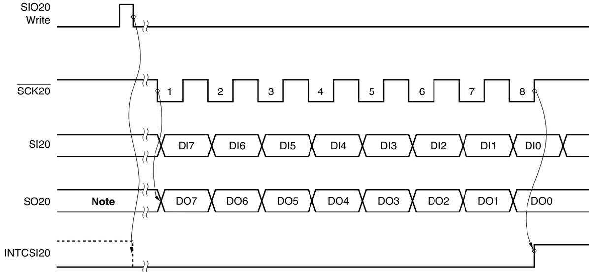
**Note** The value of the last bit previously output is output.
