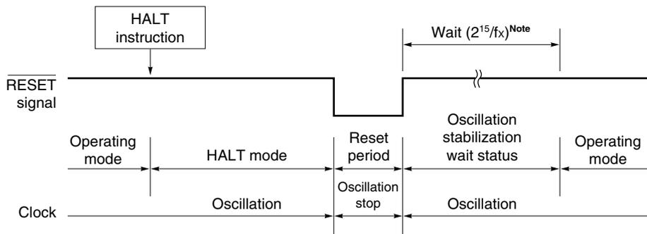
**Note** 3.28 ms (at  $f_x = 10.0$  MHz operation), 6.55 ms (at  $f_x = 5.0$  MHz operation)
