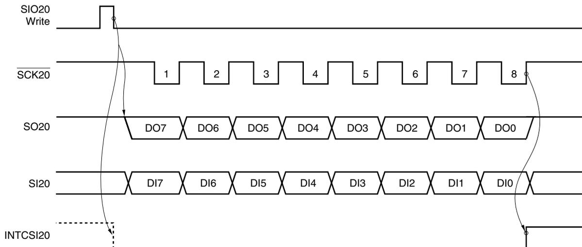
Figure 9-11. 3-Wire Serial I/O Mode Timing (5/7)
