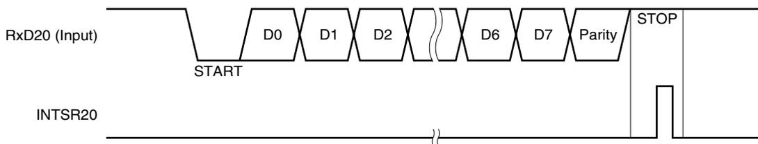
**Caution** Be sure to read receive buffer register 20 (RXB20) even if a receive error occurs. If RXB20 is not read, an overrun error will occur when the next data is received, and the receive error state will continue indefinitely.
