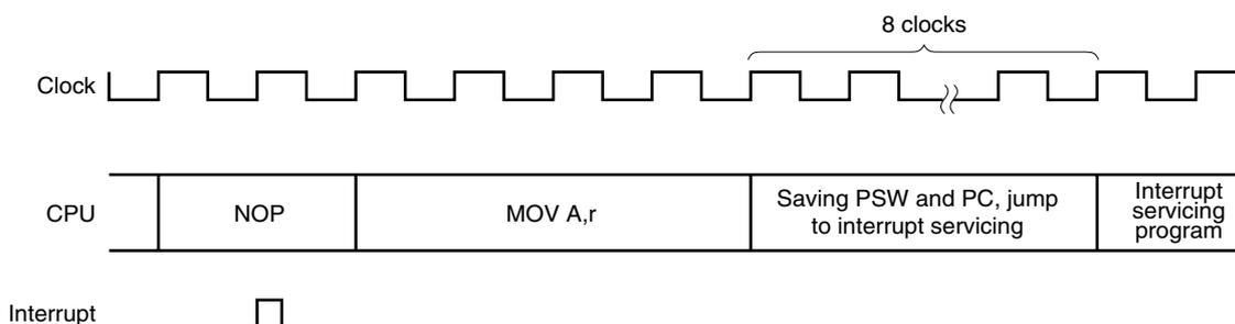
If an interrupt request flag ( $\times\times IF$ ) is set at the last clock of the instruction, the interrupt acknowledgment processing starts after the next instruction is executed. Figure 10-11 shows an example of the interrupt acknowledgment timing for an interrupt request flag that is set at the second clock of NOP (2-clock instruction). In this case, the MOV A,r instruction after the NOP instruction is executed, and then the interrupt acknowledgment processing is performed.
