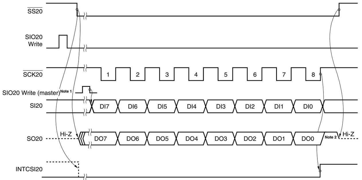
**Notes 1.** The data of SI20 is loaded at the first falling edge of  $\overline{\text{SCK20}}$ . Make sure that the master outputs the first bit before the first falling of  $\overline{\text{SCK20}}$ .
