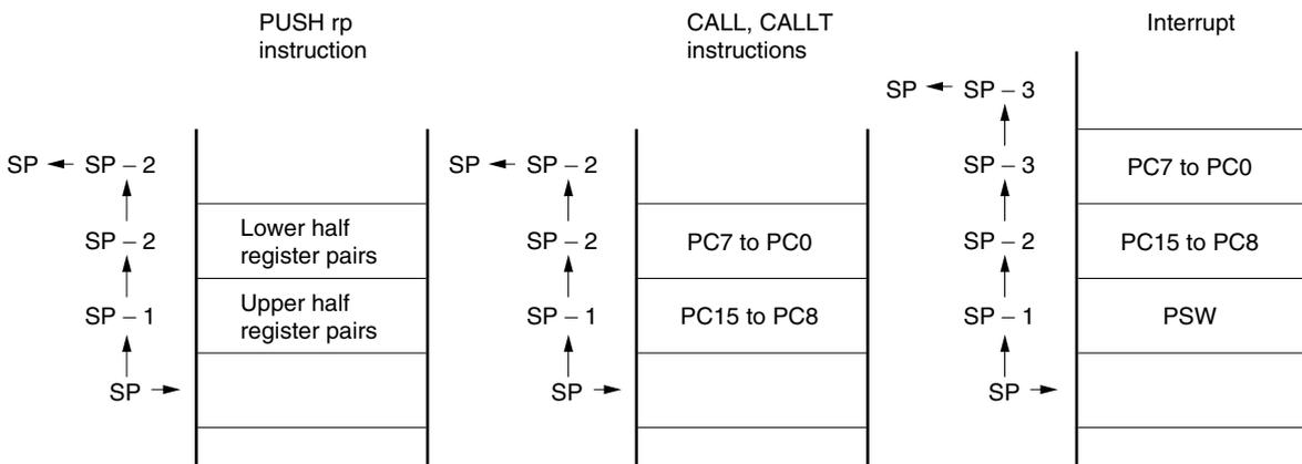
**Figure 3-13. Data to Be Restored from Stack Memory**
