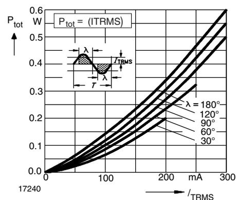
Fig. 2 - Power Dissipation 60 Hz to 60 Hz Line Operation
