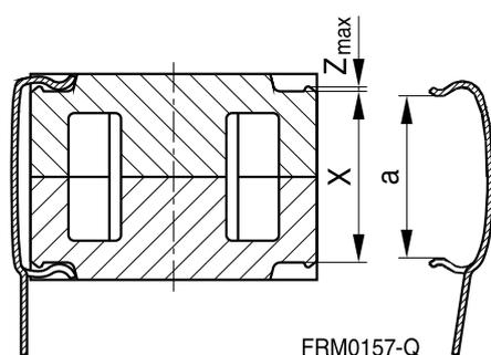
$F_{min}$ : Extension of clamp from a to  $a_2 = X_{min}$
