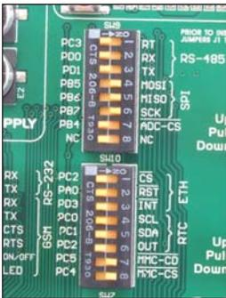
Figure 4-3: The position of DIP switches SW9 and SW10
