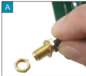
Figure 9-4: Screwing cable into antenna holder
