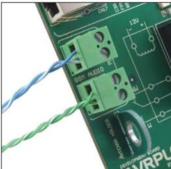
Figure 9-8: Connectors used to connect microphone and speaker
