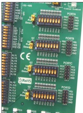
Figure 13-1: I/O ports
