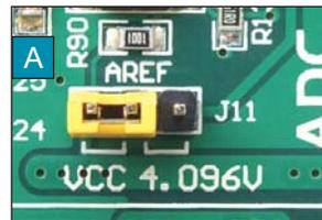
Figure 7-4: The position of jumper J11
