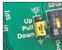
Figure 13-2: J2 in pull-down position
