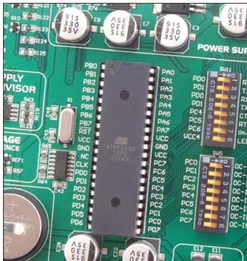
Figure 2-1: ATMEGA32 microcontroller
