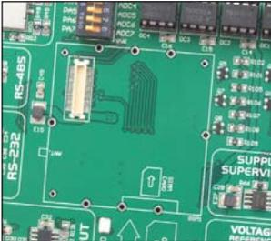
Figure 9-1: GSM connector
