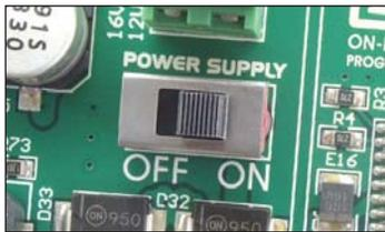
Figure 1-3: Power supply on/off switch
