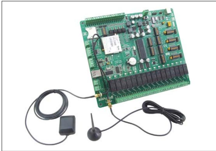
Figure 9-6: Telit's module with connected antennas
