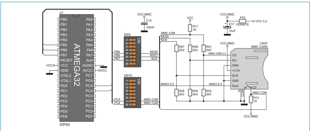
Figure 4-3: MMC/SD connector connection schematic
