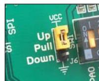
Figure 13-3: J2 in pull-up position
