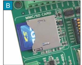
Figure 4-2: Inserting MMC/SD card
