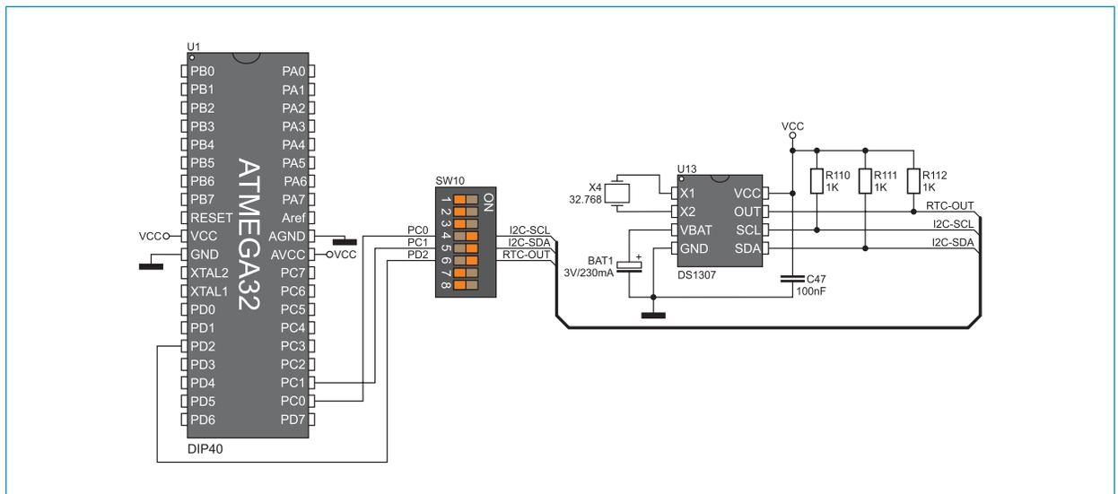
Figure 10-3: RTC module connection schematic
