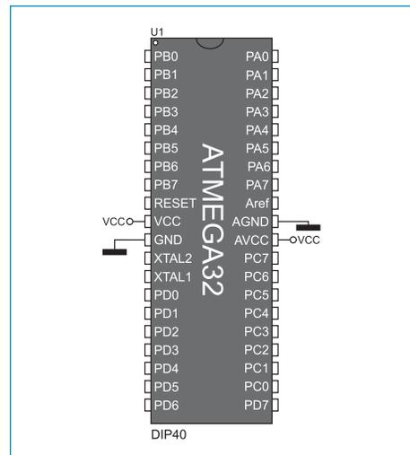
Figure 2-2: Microcontroller's pinout
