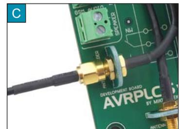
Figure 9-5: Connecting antenna
