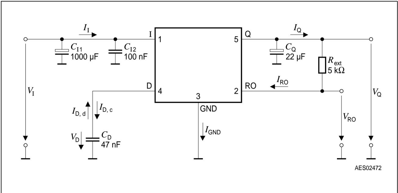
**Figure 3 Test Circuit**
