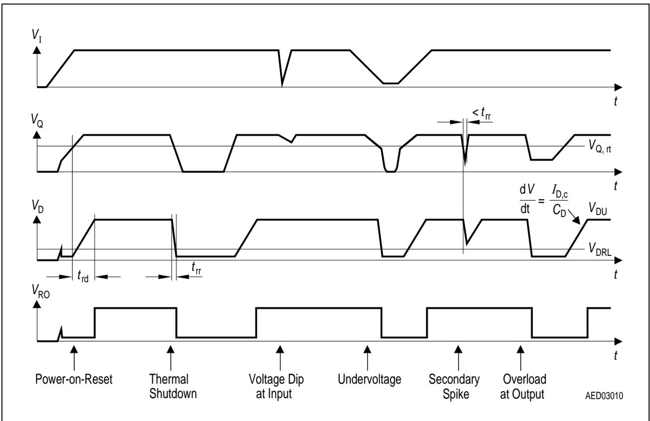
**Figure 4 Reset Timing**
