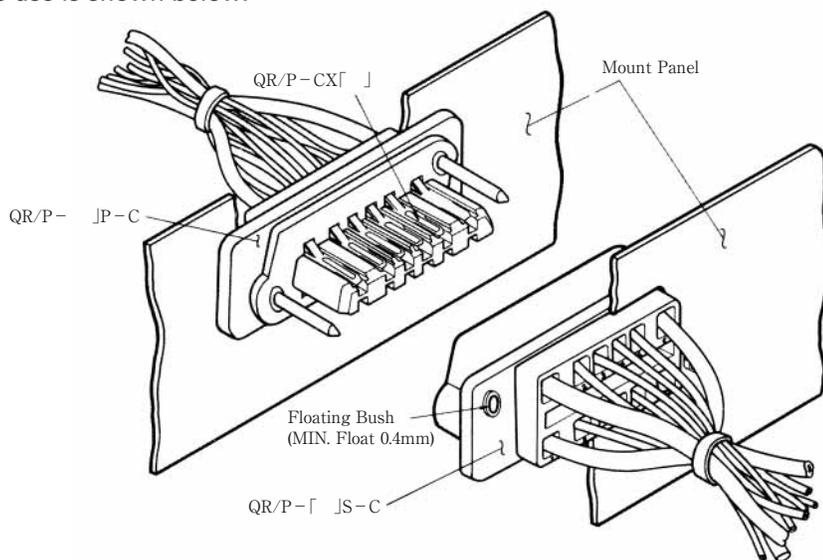
Note: Determine the combinations with the panel so that the mating clearance between the P side and S side is 2 mm or less.
