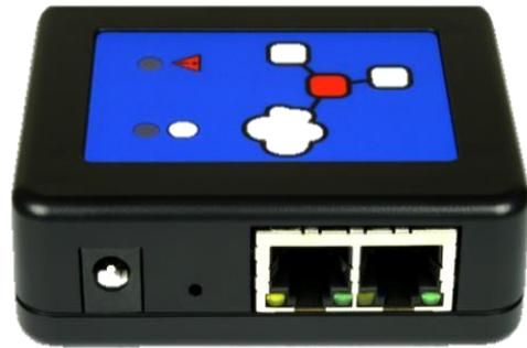
TCPCConv adds a device, which is equipped with a USB- or RS232-interface into your local area network (LAN). A typical application is the extension of a network device (i.e. a network printer) by a local peripheral device. Simply insert TCPCConv into the existing LAN connection of your device. In order to do so, TCPCConv contains 2 LAN ports, which operate as a network switch. The example below shows a typical environment, where a printer is connected to a network:
