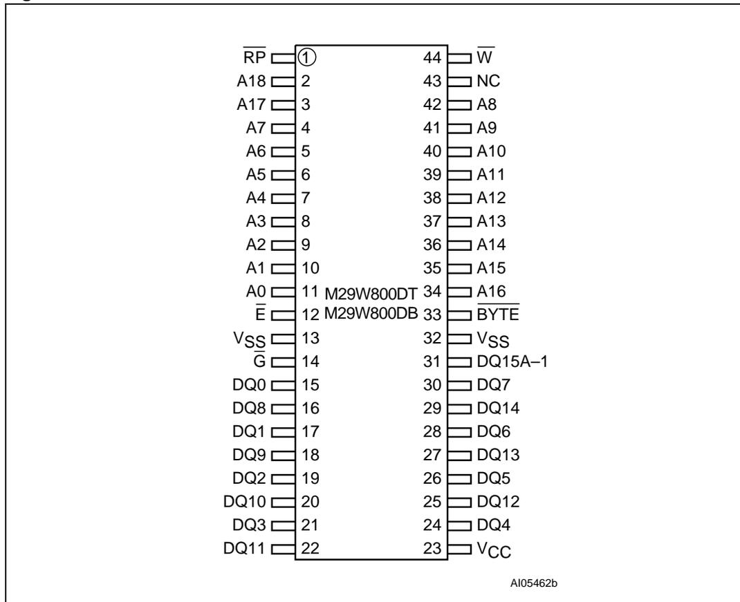
Figure 3. TSOP connections
