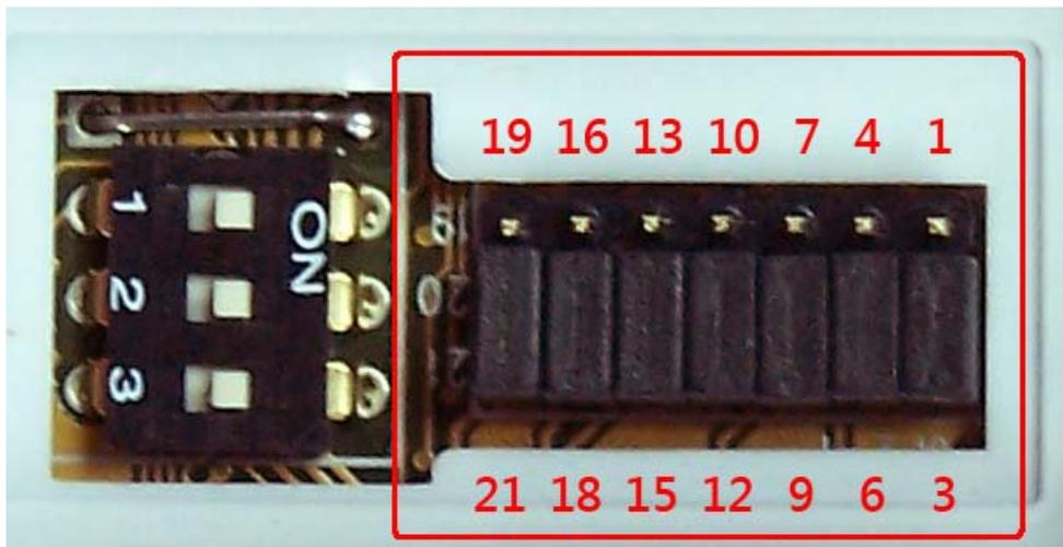
**7 x 3 header block to enable Termination and Biasing resistors**
