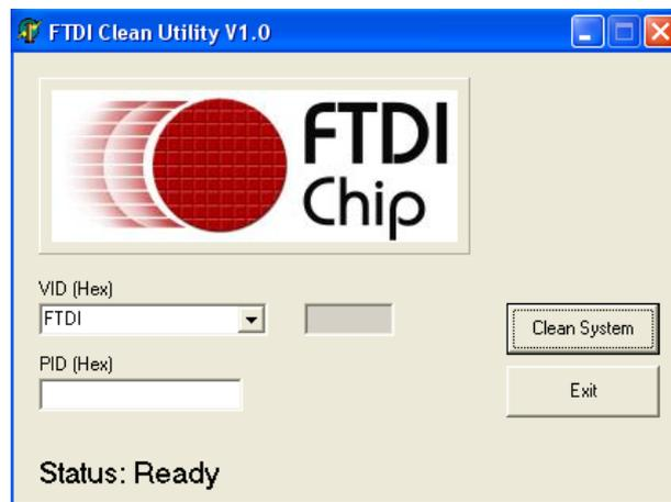
5. You need to disconnect all USB to serial Adapters from your PC, when the message below appears. Double click "OK" to start uninstalling Windows 2003/XP/2000 USB to Serial drivers.
